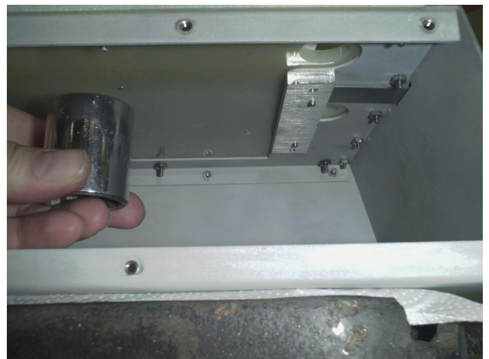
Hammering Near Left Tooling Pin Flush
